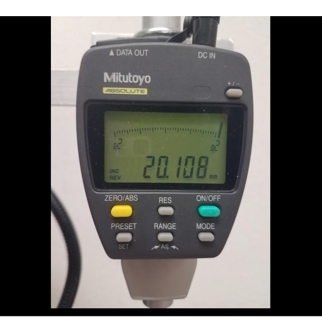
Screw this 2X Objective lens on the microscope and use it with the Digital Mitutoyo to get a Z-Reading from the culet to the table of your stone. Then use those numbers to calculate the Refractive Index of diamonds and stones with an R.I. too high to read on the refractometer.
