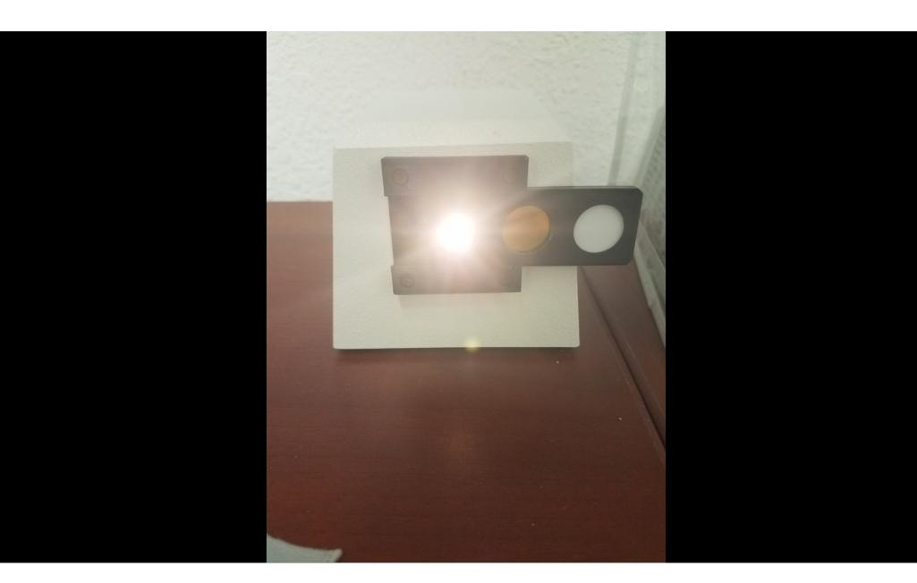
GIA Gem Instruments Duplex II Refractometer with Original Dust Cover and Paperwork
